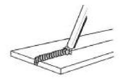
The horizontal position is performed very much the same as the flat weld except that the angle is different such that the electrode, and therefore the arc force, is directed more toward the metal above the weld joint. This more direct angle helps prevent the weld puddle from running downward while still allowing slow enough travel speed to achieve good penetration. A good starting point for your electrode angle is about 30 degrees DOWN from being perpendicular to the work piece.
