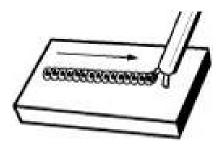
The weave bead Used when you want to deposit metal over a wider space than would be possible with a stringer bead. It is made by weaving from side to side while moving with the electrode. It is best to hesitate momentarily at each side before weaving back the other way to improve penetration.
