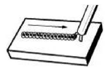
The weave bead Used when you want to deposit metal over a wider space than would be possible with a stringer bead. It is made by weaving from side to side while moving with the electrode. It is best to hesitate momentarily at each side before weaving back the other way to improve penetration.
